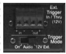
gered internally or externally. On the rear panel of the X1 is a 3-position switch that determines the trigger mode:
